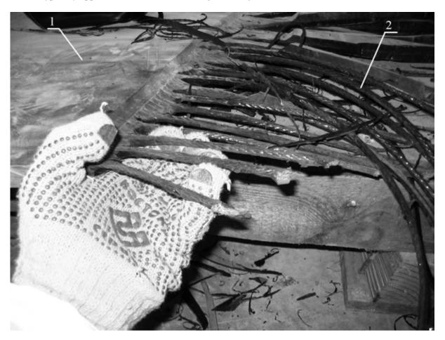
Fig. 1. General view of conveyer belt failure on Joint-Stock Company "Altyntau Kokshetau": 1 - conveyer belt; 2 - rope
