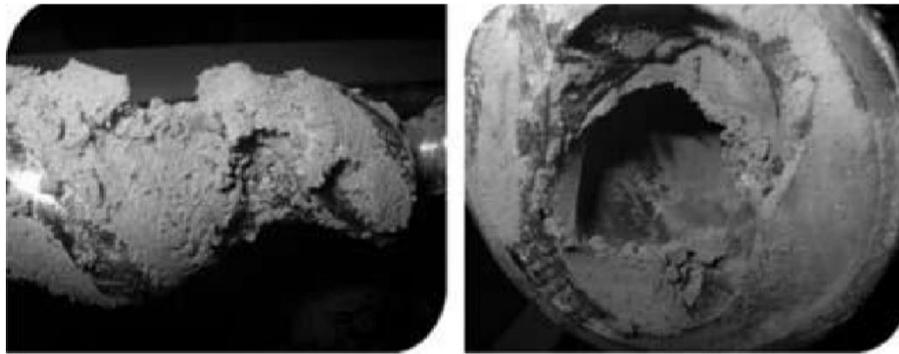
Fig. 1. Characteristics of sand plugs in the tubing string (TBS) and downhole pumping equipment (DPE) during oil production under high sand production conditions
